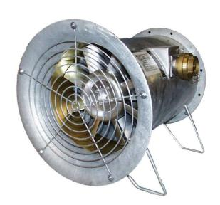
TGW-tunnel fan Size 1120, thrust 890/ 840 N, 25 kW, 70 dB(A) in 10 m, 400 °C – 1 hour.
