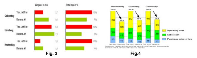
The Banana Jet produced a significantly higher airspeed in the tunnel. This is equal to a reduction in total losses of 24 - 32 % (i. e. an increase in thrust of 32 - 47 %) In all 3 tunnels further reduction in losses seemed possible if the directability of the jet had been further exploited e.g. by better countering the effect from bends, walls, lamps, etc.
