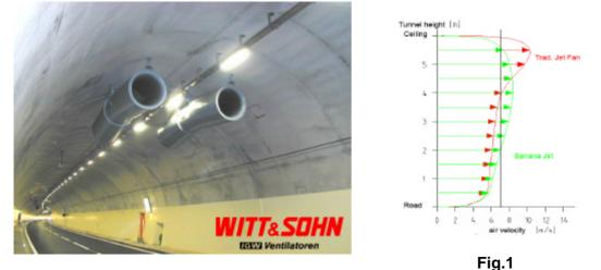
The use of Banana Jet can reduce these losses by 25 - 50 %, depending on the design of the tunnel. The physics behind this improvement is relatively straightforward:
